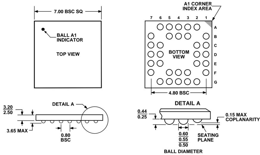
Figure 6. 32-Lead Chip Scale Ball Grid Array [CSPBGA]
